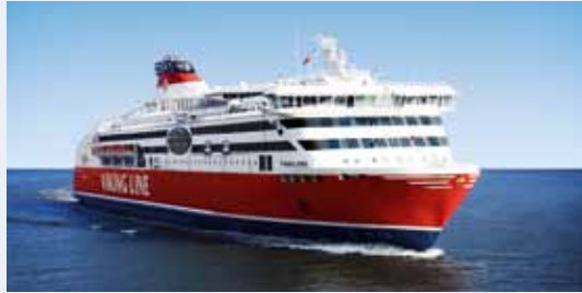
VIKING XPRS Built in 2008 • 35,918 gross registered tonnes Length 185.0 m • Ice class I A Super • 2,500 passengers 220 cars • 728 berths • Helsinki–Tallinn • Swedish flag
