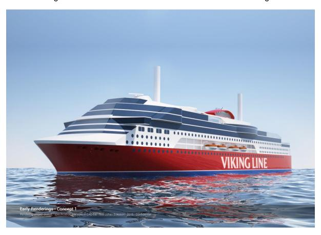
"Our intention is for the vessel to run on liquefied natural gas (LNG). We have excellent experience with this from the M/S Viking Grace, the first large LNG-powered
