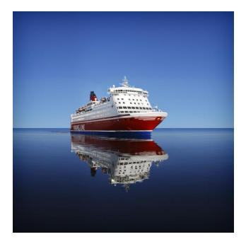
M/S Viking Isabella: Built: 1988 Split, Croatia Ice class: IA SUPER GT/NT: 34,384/19,689 Length: 169.4 meters Width: 27.6 meters Depth: 6.35 metres Speed: 20.5 knots Main engines: Wärtsilä Pielstick 23,769 kW Passengers: 2,480 Beds: 2,166 Cars: 450 Lane metres: 900 Equipped with stabilisers
